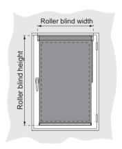
Mounting on the wing of the window Make allowance for the side distance of the fabric from the window fittings.
