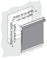
**Dimensions in the reveal**Measure the reveal exactly at the necessary mounting height.
