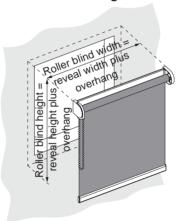
**Dimensions for face fixing**When mounting in the front of the window, allow for the necessary overhang.
