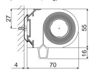
Is used in the case of roller blinds with large heights of the hanging or for fabrics of greater thickness.
