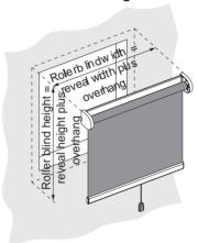
**Mounting for face fixing**When mounting in front of the window, allow for the necessary overhang.
