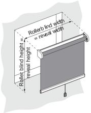
Mounting in the reveal Measure the reveal exactly at the necessary mounting height.
