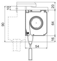
Mounting in the window jamb (with face fix bracket 33 mm)
