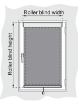
Mounting on the wing of the window Make allowance for the side distance of the fabric from window fittings.
