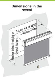
**Mounting in the reveal** Measure the reveal exactly at the necessary mounting height.
