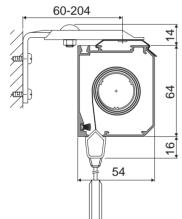
Mounting on the wing of a window (with block holder)
